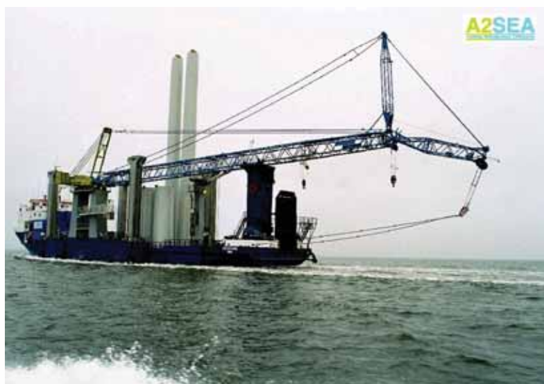
船型为风力发电机安装船舶-配有起重架以保持吊装平稳性 Ship- type WTG Installation vessel – legs add to lifting stability
