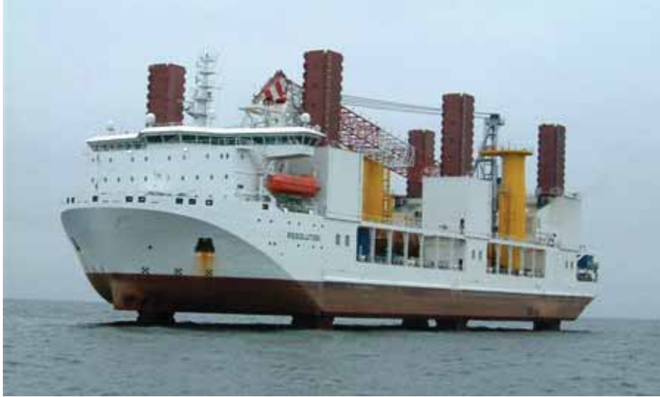
自航自升式起重机船舶-具有动态定位（DP）功能 Self-propelled jack-up crane vessel – dynamic positioning, DP
