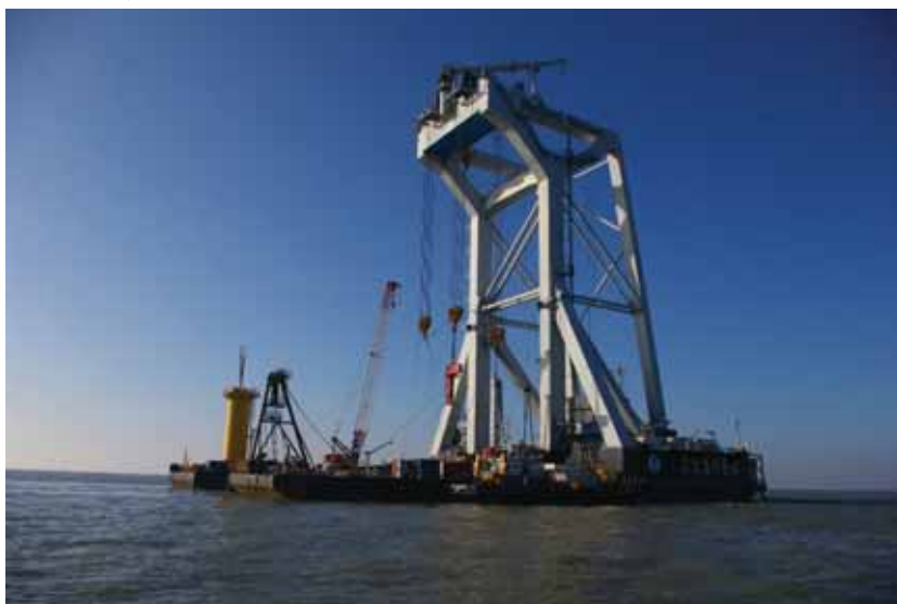
重型吊装起重机船舶 – 用于重力底座结构和分电站的安装，也可用于 风力发电机和基础的安装 Heavy-lift crane vessel – GBS, Sub-stations, but can also install WTGs and foundations
